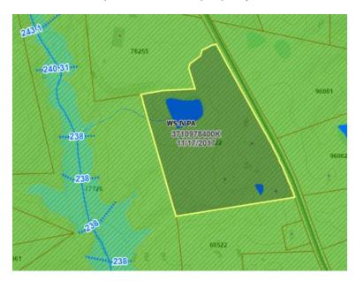
The property is located within the WS-IV Protected Area watershed district (Jordan Lake drainage) and built upon area is limited to no more than 36% without curb and gutter and the site plan shows 32.1%.
