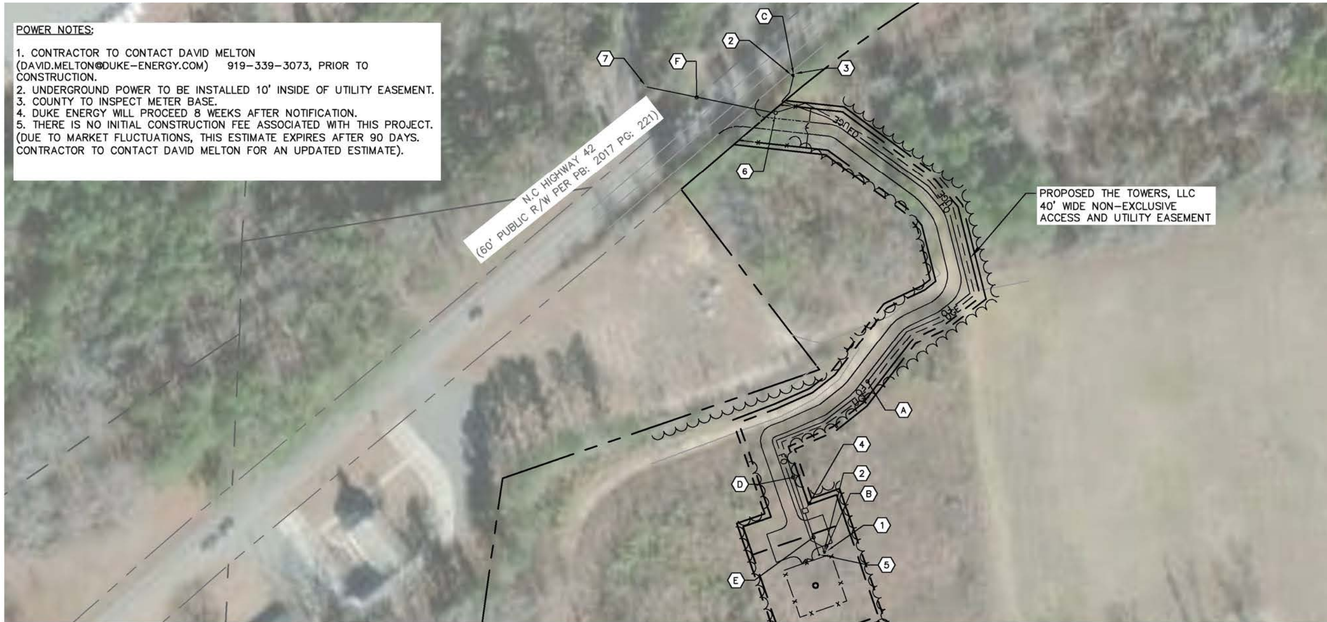
1 OVERALL UTILITY SERVICE ROUTING PLAN E2 SCALE: 1" = 100'
