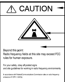
5 CAUTION-RF SIGN (YELLOW) 12" WIDE X 18" HIGH
