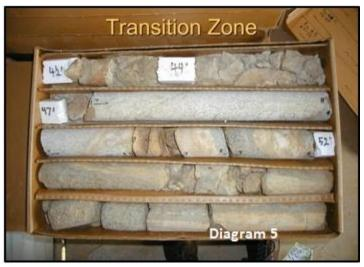
the surface to about 150 feet down. The retrieved samples show the soil, saprolite, transition zone and bedrock. The middle rows in diagram 4 show the porous transition zone, in this case at about 30 feet down. The shallow depth of the transition zone opens it up to contaminants, but the porosity transmits water well. Diagram 5 shows a detailed section of the transition zone materials, mostly made up of quartz and quartz like materials
