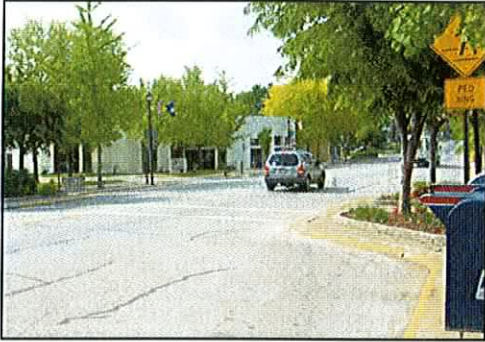
Mid-block crossings and “bulb outs” such as this one can make streets safer for pedestrians.
