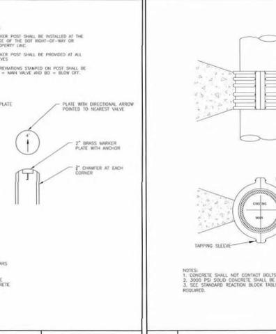
CONCRETE THRUST BLOCKING FOR VALVES AND DEAD ENDS
