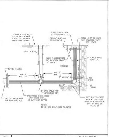
2" BLOW-OFF ASSEMBLY AT END OF WATER MAIN
