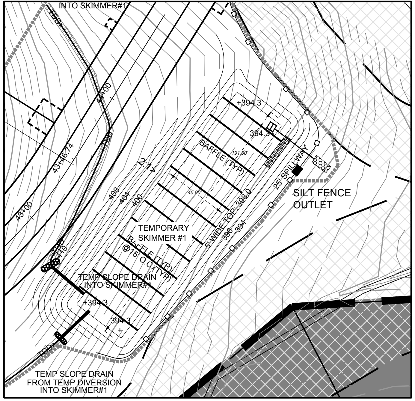
TEMPORARY SKIMMER BASIN #1 SCALE: 1"=40'
