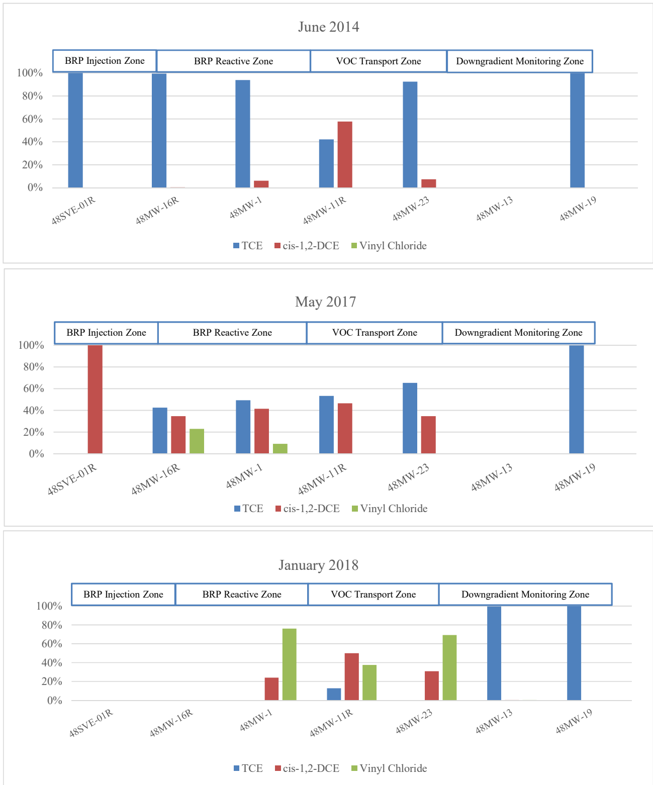
Figure 15. Molar Concentration Ratios for TCE and TCE-Daughter Products in the Shallow Aquifer Zone
