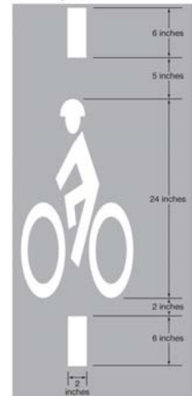
Figure 46: Pavement marking for bike actuated signal
