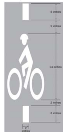
Figure 43: Pavement marking for bike actuated signal
