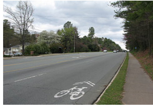
Figure 37: Shared lane marking in Chapel Hill
