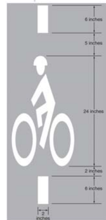
Figure 41: Pavement marking for bike actuated signal
